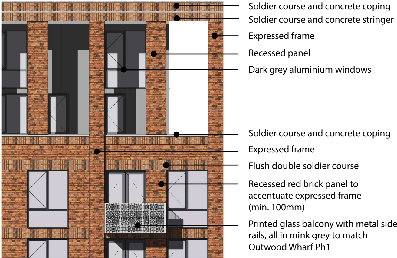
Typical Duplex Elevation - Gaythorn Street
