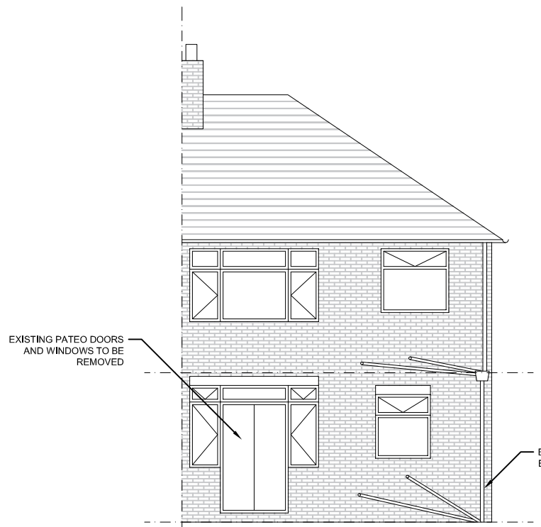
EXISTING REAR ELEVATION
